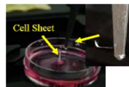
Force measurement for cell sheet adhesion (UAT)
