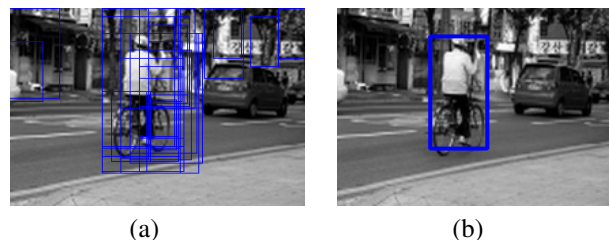
Fig. 4 Merge processing: (a) Before merging, and (b) after merging.
