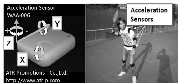
Figure 1. An acceleration sensor and the state that player wore the acceleration sensors.
