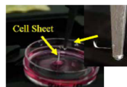
Force measurement for cell sheet adhesion (UAT)
