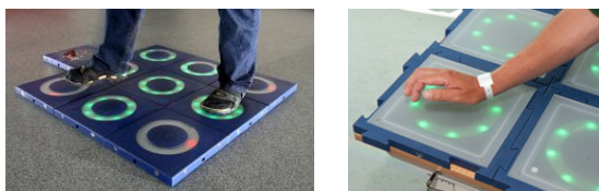
Fig. 1. Modular tiles used for feet or hands interaction.
