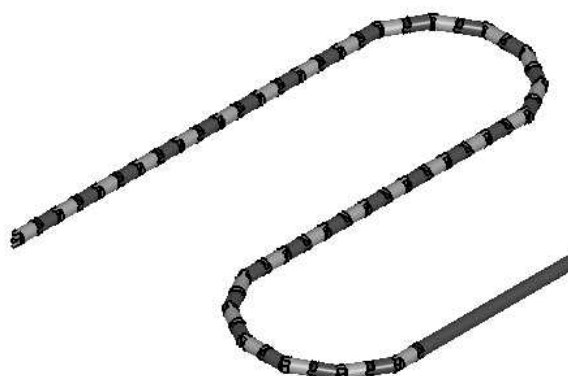
Fig.2. Flexible shaft composed of short links
