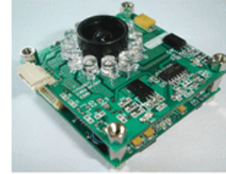
Fig. 5. localization sensor module (Hagisonic co.)
