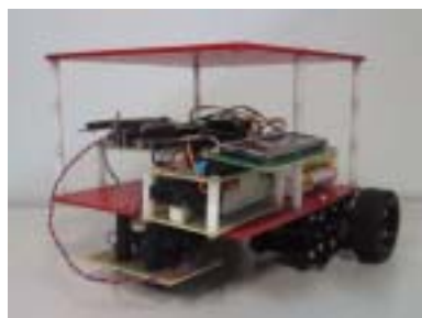
(a)PSD module and Tire type line tracer (A)
