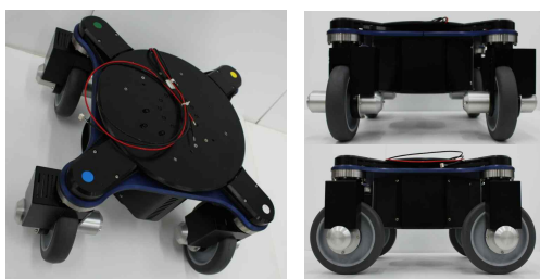
Fig.7. Prototype of Omni-directional Mobile Module
