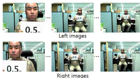
Fig.6. test image set with real distance value (0.5~3.5m)
