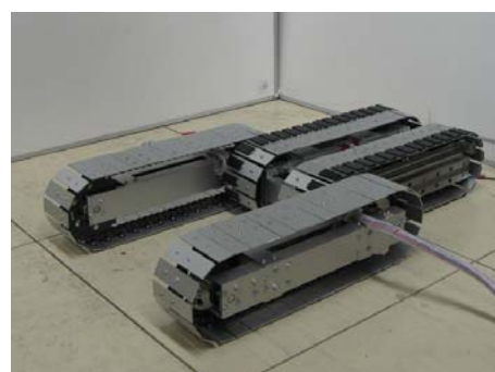
Fig.7. Overview of expanding side crawler
