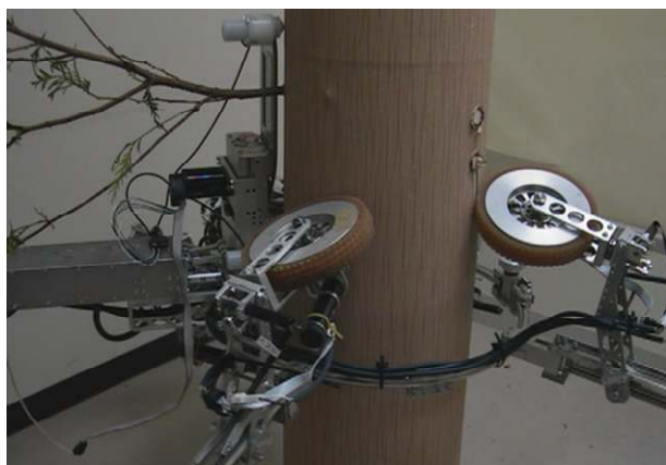
Fig. 8 Pruning experiment with pruning robot
