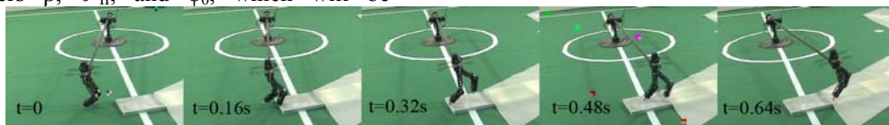
Fig. 9 Image sequence extracted from video of a single step-up perturbation experiment ( h_r^{\max}=25\text{mm} )
