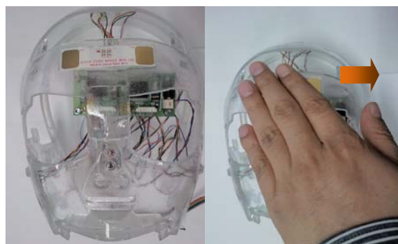
Fig. 4 Touch operation on the touch sensor pad
