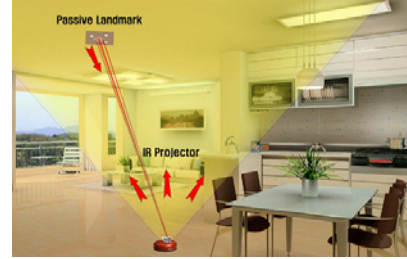
Fig. 4. Indoor localization system (Hagisonic co.)
