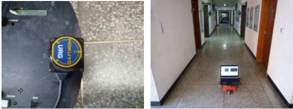
Figure 1. Laser range finder & Indoor environment
