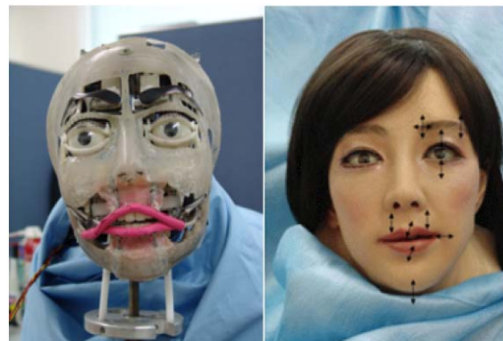
Fig. 2 Ever-2 Head : inner structure and face variety of movements can not be guaranteed. Therefore, various facial expressions are critical problems in the android robot.
