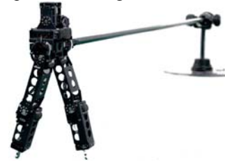
Fig. 8 Planar Bipedal Robot Stepper-2D with Point Foot.
