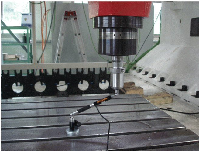
Fig. 6. Calibration experiment using a ball-bar.
