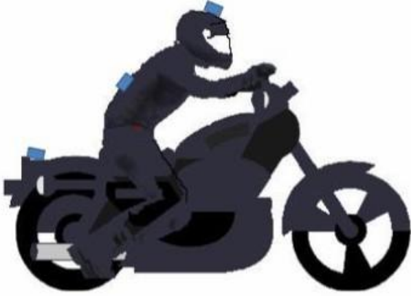
Fig. 2. Sensor placement concept for blind-spot monitoring and forward- collision alert.
