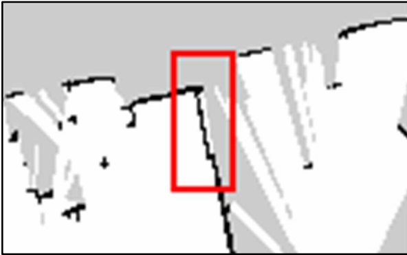
Fig. 1. A region of the original map with odometry caused artifact (obstacle-free space behind the wall).
