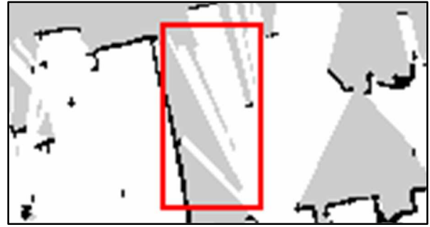
Fig. 3. A region of the original map with highlighted space between distinct laser rays.
