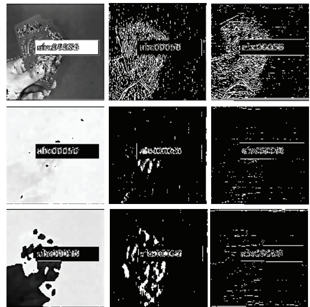
Fig. 4. 1HL (upper & center) and 1LH (upper & right) elements for Y element (upper & left), 1HL (middle & center) and 1LH (middle & right) elements for Cr element (middle & left), and 1HL (lower & center) and 1LH (lower & right) elements for Cb element (lower & left) obtained from input image (Fig. 3).
