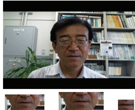
Fig. 1. Face image (upper), lower part of face image before (lower & left) and after (lower & center) standardization of size, and mouth-area image extracted (lower & right).
