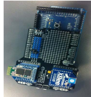
Figure 2. Arduino Uno with beeshielded Bluetooth and Xbee.
