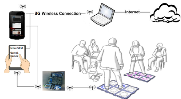
Figure 1: The concept connects modular interactive tiles with radio via a board with XBee and Bluetooth to Android tablets and smart phones, which can connect to the Internet (e.g. for storing database). Players can choose games and player IDs on the smart device(s) and monitor their performance on the smart device(s).
