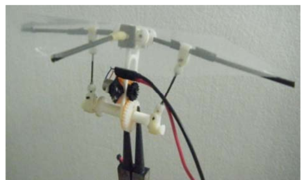
Fig. 6. Third prototype is setup with the second design of wing structure. Wing is made from plastic sheet with a wingspan of 15 centimeters.
