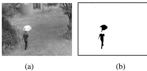
Fig. 2. Example of the performance: (a) Original image, (b) the moving object detection followed by the morphological operation.
