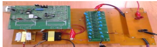
Fig. 3. The boosting circuit for 20KVDC arc discharge.
