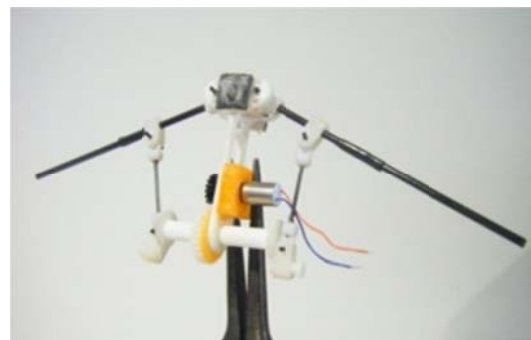
Fig. 3. The third generation of mechanism design for the flapping-wing robot.
