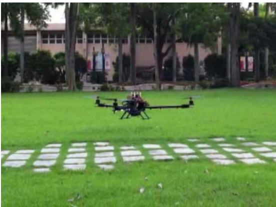
Fig. 9 Outdoor flight test of the tri-rotor flying robot with KK multicopter installed
