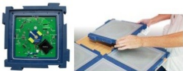
Figure 1: Left: The interior of the modular interactive tiles. Right: A tile playfield being assembled.
