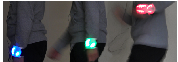
Fig. 6. The developed device in use. LED lights up in synchronization with the heart beat, and the color changes according to the calculated heart beat rate.
