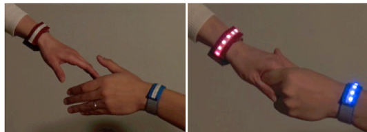
Fig. 3. The six full color LEDs are installed in the bracelet, which are lit up when handshake occurs.
