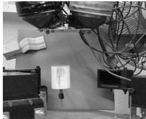
Fig. 6. Photograph of the levitated hand that is carrying a transistor
