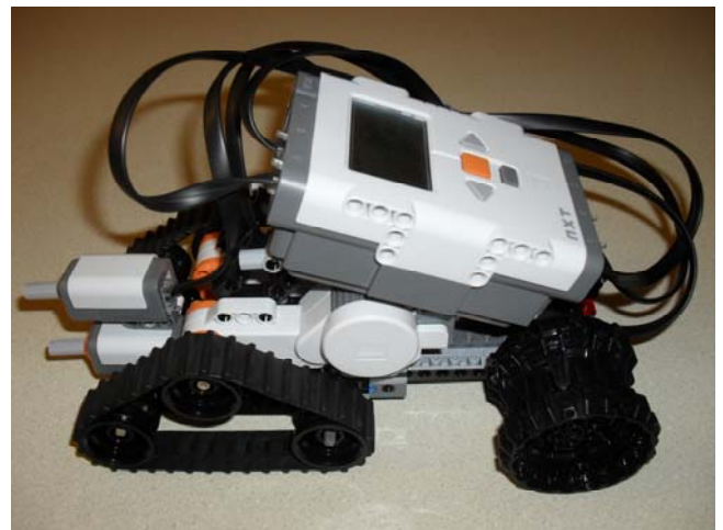
Fig. 1. Picture of one of the robots that was used for testing the system. This robot has its second bump sensor set at the lowest setting (directly above the lower sensor). Other robots had their sensors at higher settings.
