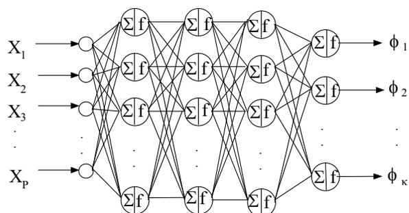
Fig.1 Architecture of revised GMDH-type neural network
