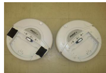
Fig. 6. Two iRobot Create using in our experiments. The left Create is with black label, while the right one is regular Create.
