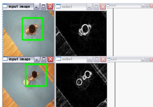
Fig.8. Detect person by Hough Transform and Brightness Histogram
