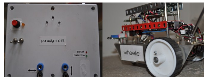
Figure 11: Proof of concept - Control Module (L) and Wireless robot (R)
