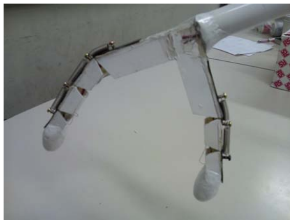
Fig. 4. Test model of wire-driven two-fingered robotic system
