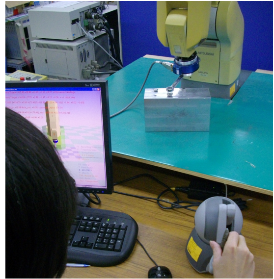
Fig. 2: The user applies the proposed system to manipulate the real robot manipulator via a haptic input device and 3D graphical environment.
