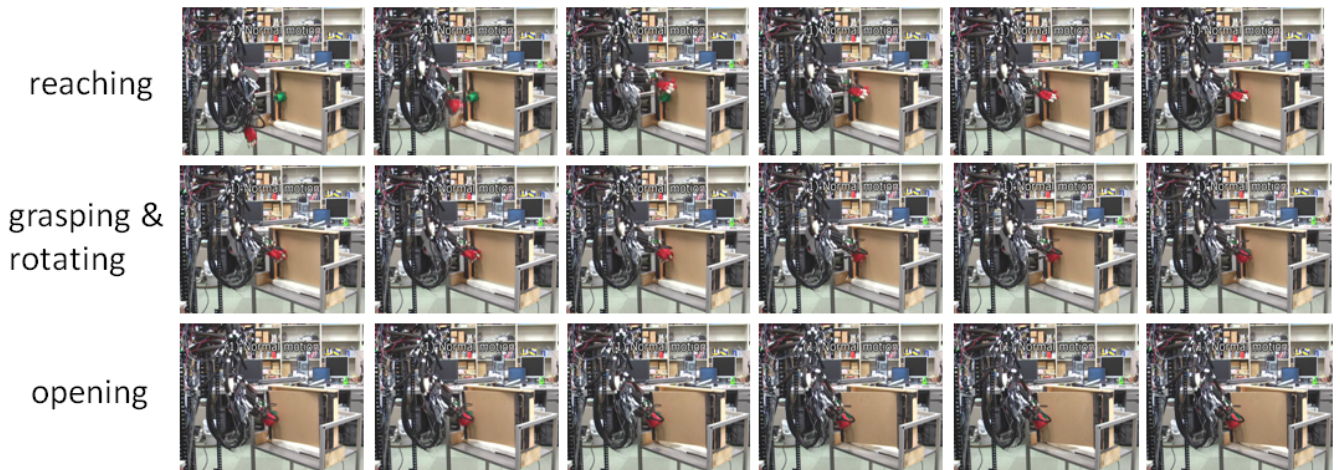
Fig. 5. The execution of the door-opening task. The developed musculoskeletal robot arm can adaptively grasp and rotate the door knob, and open the door by exploiting its morphological computation.
