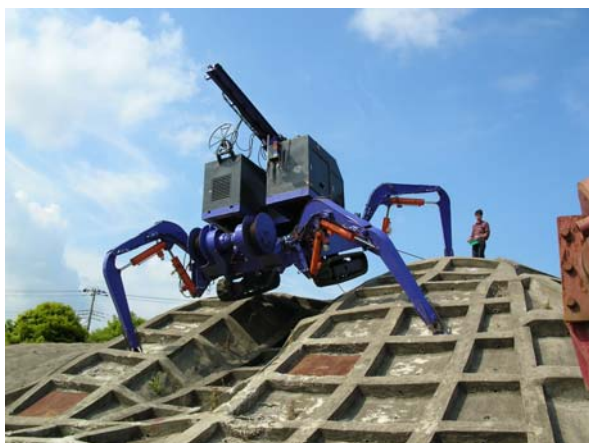
Figure.23: Walking with tether on slope
