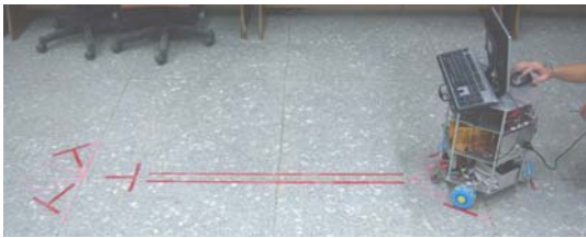
Fig.10. Test of moving distance after motor stop for different motor speed
