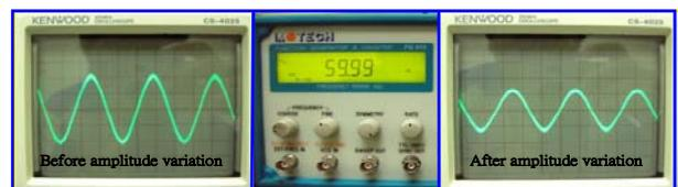
Fig. 2. The wave form of function generator by oscilloscope display.
