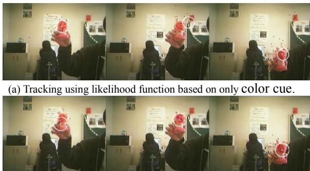
(b) Tracking using likelihood function based on color and motion
