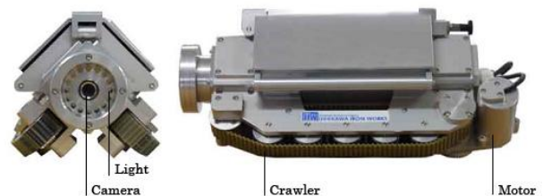
Fig.1. Structure of the inspection robot
