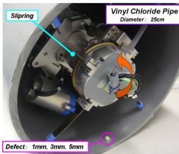
Fig.11. Voltage change measurement in the pipe
