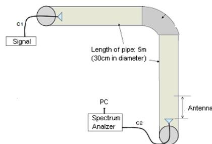
Fig.1. Wireless communication property measurement inside the steel pipe
