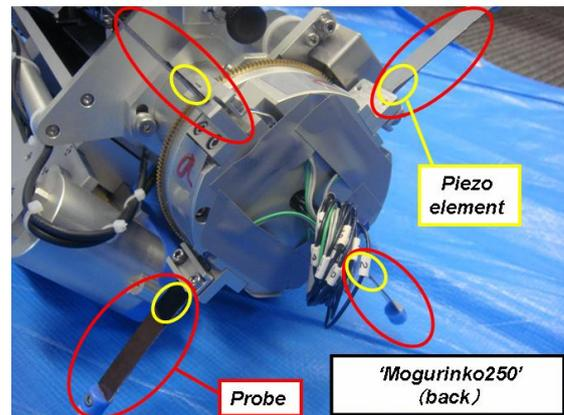
Fig.9. Rotating probe
