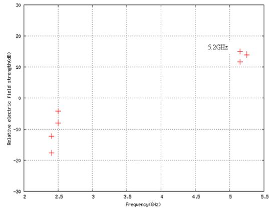
Fig.5. Wireless communication result in ceramic pipe
