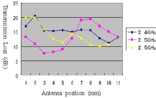
Fig.2. Transmission loss measured in steel pipe (2.4 GHz)
