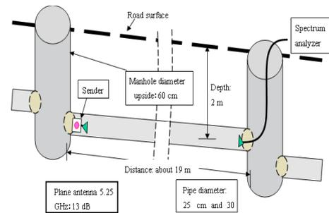
Fig.6. Transmission loss measurement system
