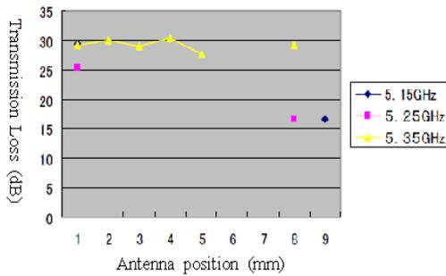
Fig.3. Transmission loss measured in steel pipe (5.2 GHz)
