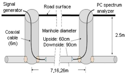
Fig.4. Wireless communication property measurement in the ceramic pipe
