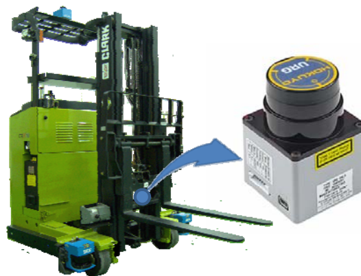
Fig.1. LRF is set up at forklift AGV
