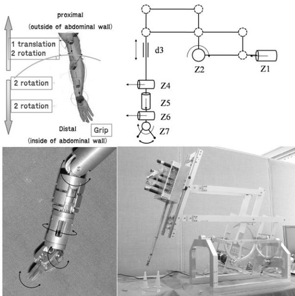
Fig.1. configuration of the manipulator
