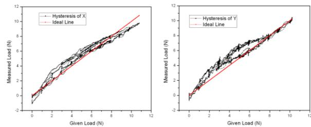
Fig.5. Hysteresis curve of x and y-axis force
