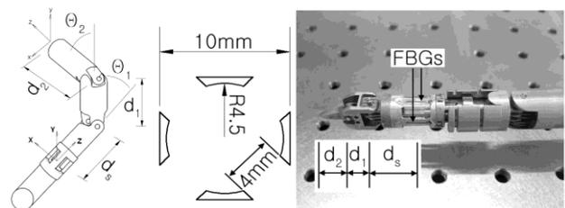
Fig.2. Sensor kinematics, cross section of sensor and developed sensor
