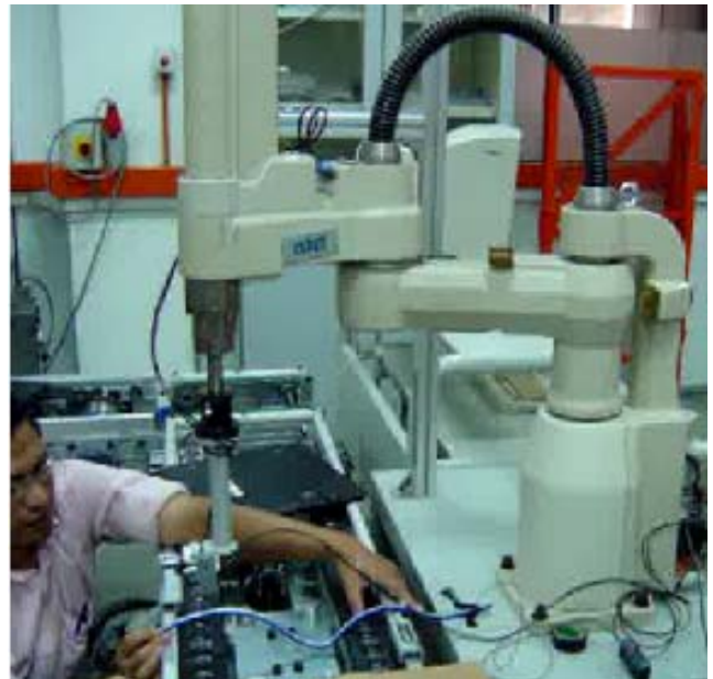
Fig.1 Fuzzy Sweeping Radius with ADEPT SCARA Robot Implementation
