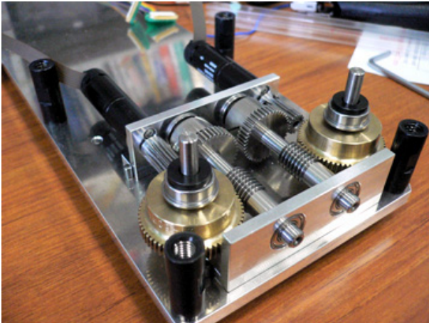
Fig.5. Wire Take-up Mechanism
