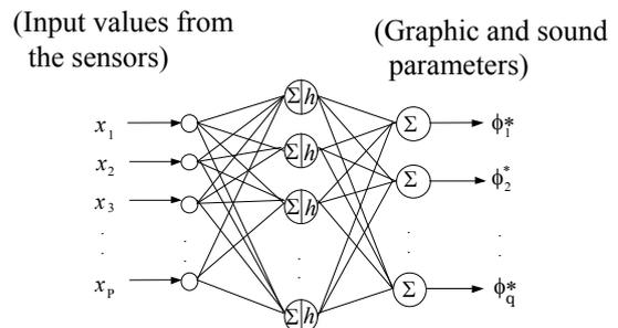
Fig.4 Architecture of the revised RBF network (2)
