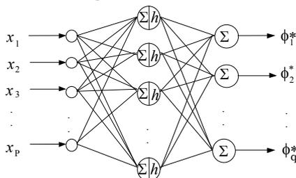
Fig.1 Architecture of the revised RBF network (1)
