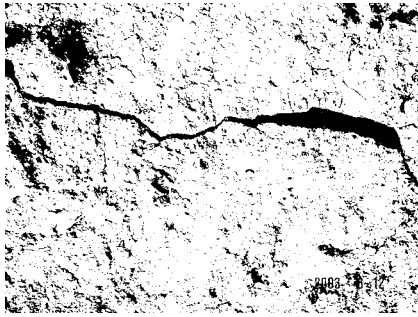
Fig.5. Result of global thresholding from Fig.4.
