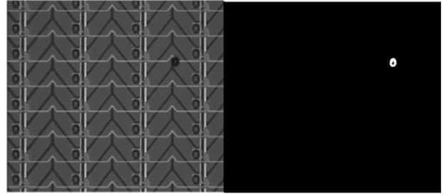
Fig.2. Tested image with defective pixels and resultant image.
