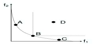
Figure 1: The concept of dominance in multi-objective optimization. Assuming that both  $f_1$  and  $f_2$  are to be minimized, D is dominated by B since B is better than D when measured on all objectives. However, A, B and C are nondominated since none of them is better than the other two when measured on all objectives.
