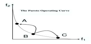
Figure 2: The Pareto Operating Curve. Solution B can be the best solution for a specific level of trade-off between objective function  $f_1$  and  $f_2$  at time t. When the required level of trade-off changes, this solution may need to move along the curve to become, for example, solution A or C.
