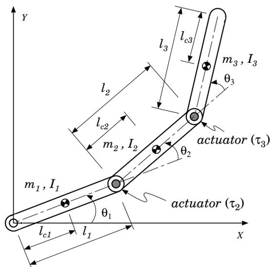
Figure 1: The three-DOF manipulator system
