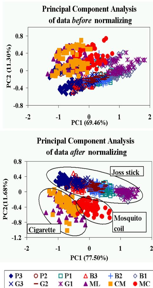
Fig.3. Two main components of the experimental data using the PCA.
