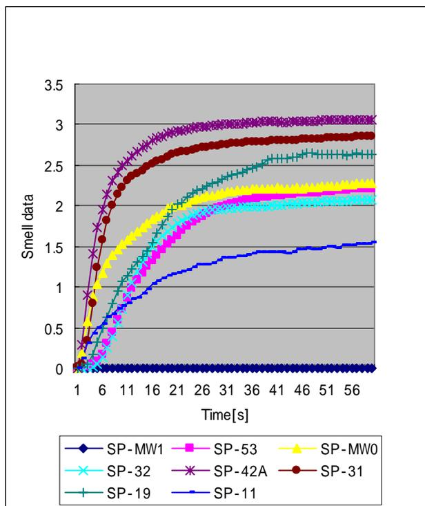
Fig.2 Time series data from some sources of fire in the experiment.
