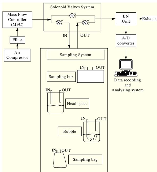
Fig. 1 Schematic diagram of the electronic nose system.
