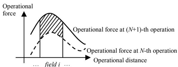
Fig. 2 Profiles (operational force)
