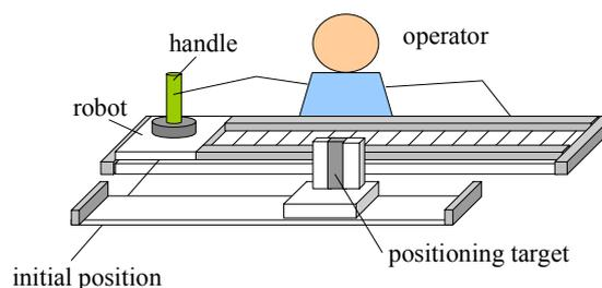
Fig. 1 A 1-DOF power-assist robot
