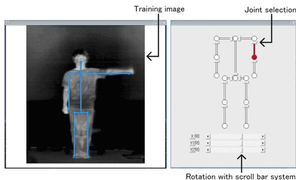
Fig.2. Manual model fitting
