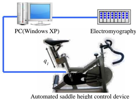
Fig. 1 Automatic saddle height control system muscles
