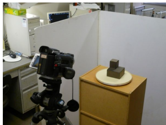
Fig. 4. Experimental setup: A digital video camera and a turntable on which an object is placed. The turntable is given turns manually for multiple views by the camera.
