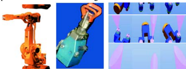
Fig. 4 : Robot selected for spray painting with the end-effector and the tool adapted in the simulation
