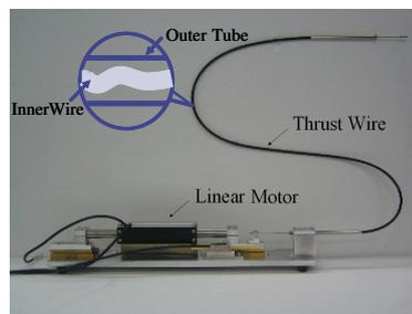
Fig. 5. Schematic diagram of flexible actuation system
