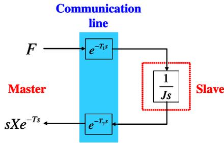
Fig. 7. Example of time delayed telehaptics system
