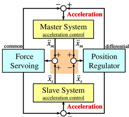
Fig. 2. Robust bilateral control system
