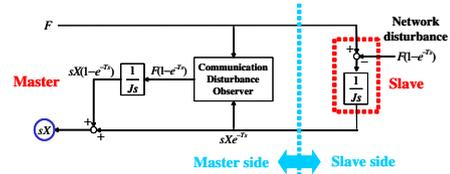
Fig. 9. Schematic diagram of time delay compensation
