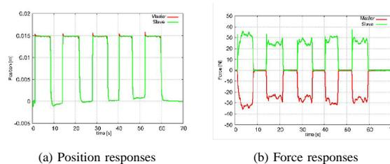
Fig. 3. Experimental results on acceleration-based bilateral control
