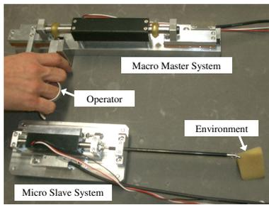
Fig. 10. Haptic forceps robot
