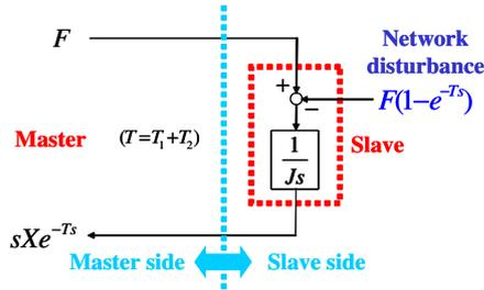
Fig. 8. Concept of network disturbance (ND)
