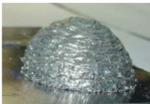
Fig. 9. The fabricated metallic Half ball part by the proposed pre-placed powder based RT system.
