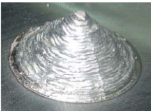
Fig. 10. Another fabricated RT part by the proposed pre-placed powder based RT system.
