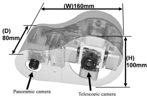
Fig. 1 Double-lens tracking-camera.
