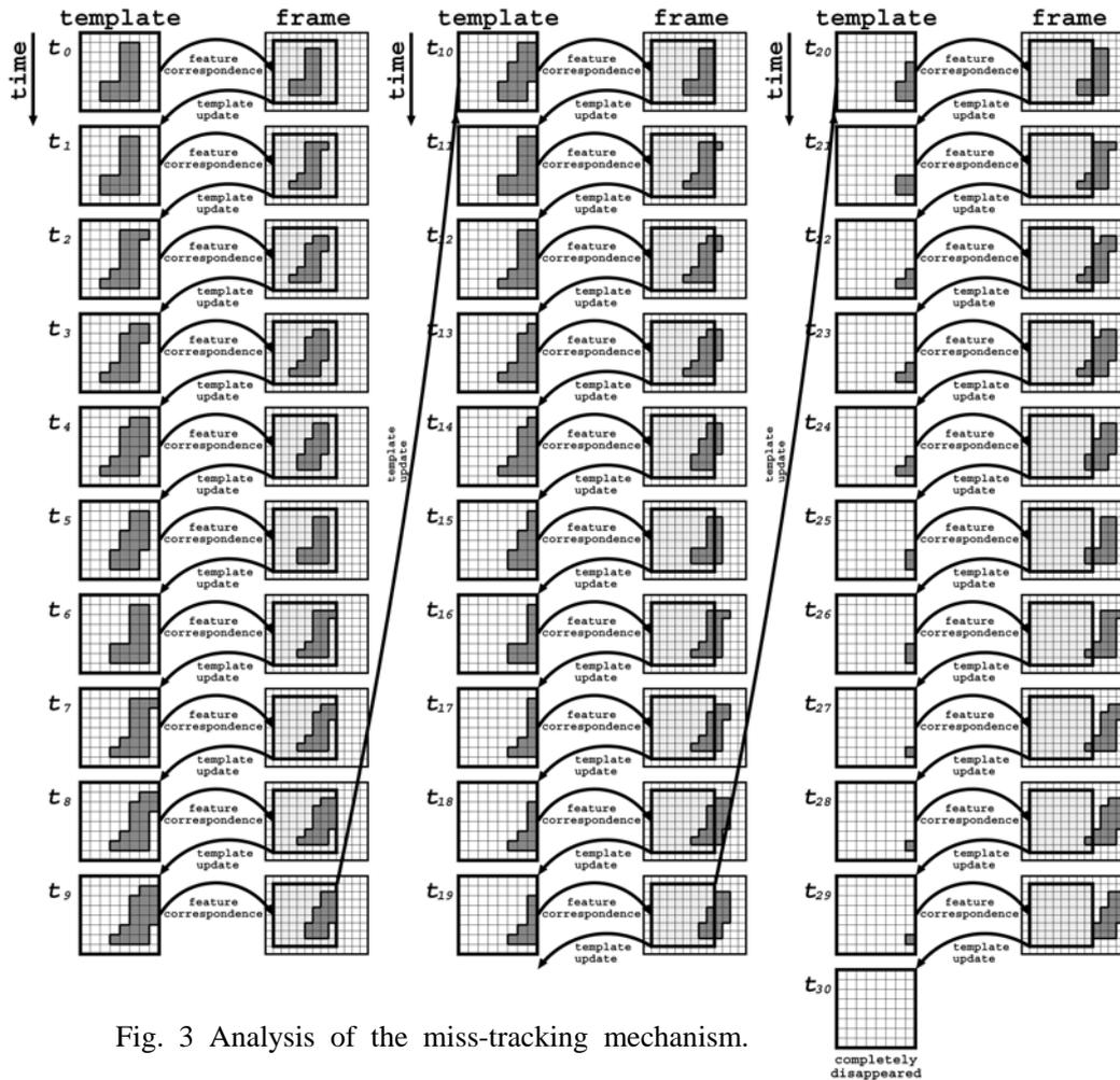
Fig. 3 Analysis of the miss-tracking mechanism.
