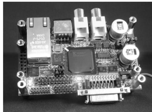
Fig. 2 FPGA board.
