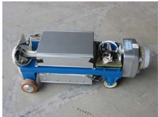
Fig.16 Moving Robot for drainpipe
