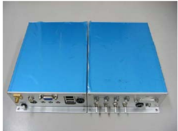
Fig.15 Compact Radio communication system Fig.13-15 shows the compact radio communication system and battery system.
