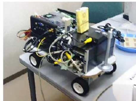
Fig. 10 Pipe Inspection Test Robot system
