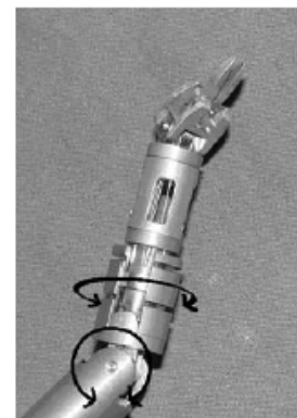
Fig.1. Two degrees-of-freedom elbow motion
