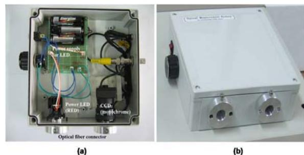
Fig. 5. Optical measuring system of this tactile sensor system; (a) The interior, (b) The exterior
