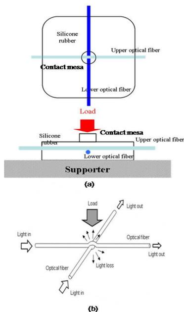
Fig. 2. (a) Structure of the taxel, (b) the microbending effect of the optical fibers in the silicon rubber.
