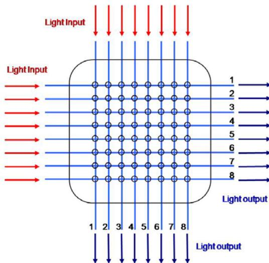
Fig. 7. Schematics of the tactile sensor using microbending fiber optic sensors with the fabric structure
