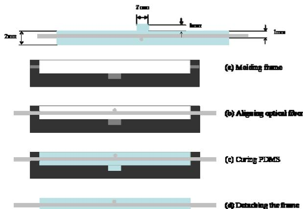
Fig. 3. Dimension of the taxel and its fabrication.
