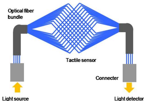
Fig. 8. Schematic for the tactile sensing system
