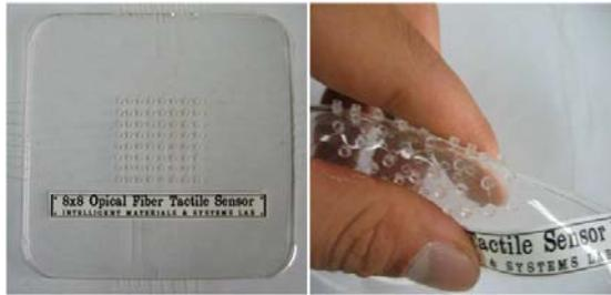
Fig. 9. Fabricated prototype tactile sensors and its flexibility
