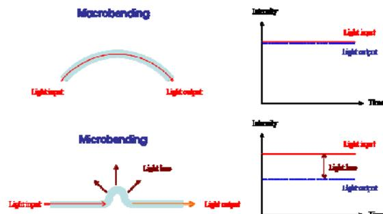
Fig.1. Microbending effect of the optical fiber.
