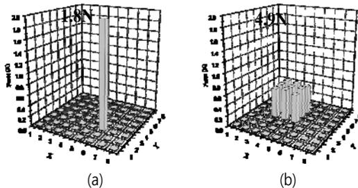
Fig. 10. Experimental results of the tactile sensor; (a)point load detection, and (b)distributed load detection.
