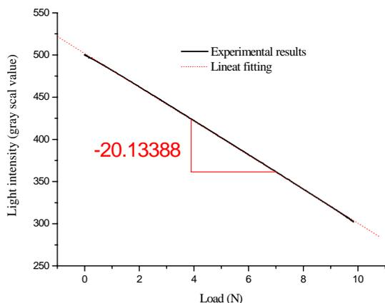
Fig. 6. Experimental verification of the prototype taxel.
